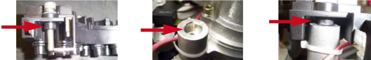
5. Fit the new rectifier by hand, ensuring all 4 insulation bosses seat correctly in the rear end housing, as shown in 4 above.
