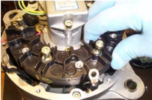
6. Fit new insulation washer, steel washer, spring washer and capscrew (items 6, 3, 5, 4). Screw down the 4 new screws and torque to 7Nm. (Also see drawing on page 3)
